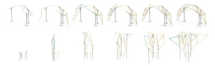
Fig. 12. The first row visualizes the assembly sequence of the ARCH model from [Bruun et al. 2022] by using 3 static supports and assembling 4 bars per step. The second row visualizes the assembly sequence of the MYCOTREE model from [Lee 2018] using 3 dynamic holdings and assembling 4 bars per step. All bars share the same material properties R = 10 mm, D = 5.8 kN/ $m^3$ , E = 12.9 GPa, G = 4.6 GPa.
