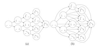
Fig. 4. (a) The state graph of a four-part assembly, when only one bar is installed at a time (h = 1). (b) The state graph of the same four-part assembly, when at most two bars can be installed at a time (h = 2). Both graphs share the same nodes, but the state graph in (b) has more edges than the state graph in (a).
