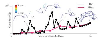
Fig. 9. Installing a 39-part bridge structure [2021] by assembling at most 1 (black) or 5 (magenta) bars per step. The plot shows the compliance of the two sequences over the number of installed bars. The 1-Bar sequence is computed using our *z*-LANDMARK solver, and the 5-Bar sequence is computed using our HOLISTIC solver. All bars have the same material properties R = 10 mm, D = 12.7 kN/ $m^3$ , E = 2.07 GPa, G = 0.89 GPa.
