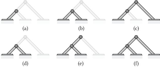
Fig. 5. Each of the substructures in (a), (b), and (c) has the lowest compliance among other substructures with the same number of bars. However, there is a bar in (b) that is not in (c). Directly linking (a), (b), (c), and (f) does not form a temporal coherent assembly sequence. A globally optimal assembly sequence is defined by substructures (a), (d), (e), and (f).
