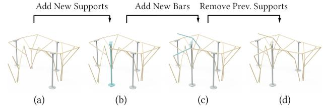
Fig. 8. New supports are first installed in (b) before the new bars are installed in (c). Supports that are no longer needed are removed in (d). Newly introduced bars or supports are highlighted in cyan.
