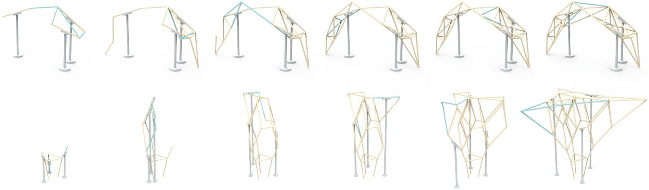
Fig. 12. The first row visualizes the assembly sequence of the ARCH model from [Bruun et al. 2022] by using 3 static supports and assembling 4 bars per step. The second row visualizes the assembly sequence of the MYCO TREE model from [Lee 2018] using 3 dynamic holdings and assembling 4 bars per step. All bars share the same material properties  $R = 10$  mm,  $D = 5.8$  kN/m<sup>3</sup>,  $E = 12.9$  GPa,  $G = 4.6$  GPa.
