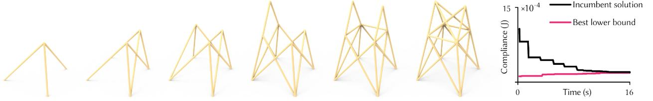
Fig. 6. An assembly sequence computed using our BnB solver for constructing a 24-bar TOWER model [Fox and Schmit Jr 1966]. The sequence contains 6 assembly stages with non-uniform step sizes, where at most 5 bars are installed at a time. The right plot shows the assembly cost of the incumbent solution and the current best lower bound over the computational time. A global minimum is found when these two lines meet.
