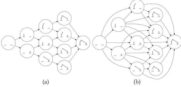
Fig. 4. (a) The state graph of a four-part assembly, when only one bar is installed at a time ( $h = 1$ ). (b) The state graph of the same four-part assembly, when at most two bars can be installed at a time ( $h = 2$ ). Both graphs share the same nodes, but the state graph in (b) has more edges than the state graph in (a).
