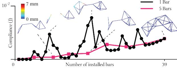
Fig. 9. Installing a 39-part bridge structure [2021] by assembling at most 1 (black) or 5 (magenta) bars per step. The plot shows the compliance of the two sequences over the number of installed bars. The 1-Bar sequence is computed using our z-LANDMARK solver, and the 5-Bar sequence is computed using our HOLISTIC solver. All bars have the same material properties  $R = 10$  mm,  $D = 12.7$  kN/m<sup>3</sup>,  $E = 2.07$  GPa,  $G = 0.89$  GPa.
