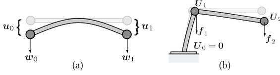
Fig. 3. (a) A deformed bar with a deformation vector  $\mathbf{u} = [\mathbf{u}_0^T, \mathbf{u}_1^T]^T$  and an external force vector  $\mathbf{w} = [\mathbf{w}_0^T, \mathbf{w}_1^T]^T$ . (b) A deformed incomplete substructure, whose leftmost joint is anchored to the ground, so  $\mathbf{U}_0 = \mathbf{0}$ . Its global deformation vector is  $\mathbf{U} = [\mathbf{U}_1^T, \mathbf{U}_2^T]^T$  and its global external force vector is  $\mathbf{F} = [\mathbf{f}_1^T, \mathbf{f}_2^T]^T$ .
